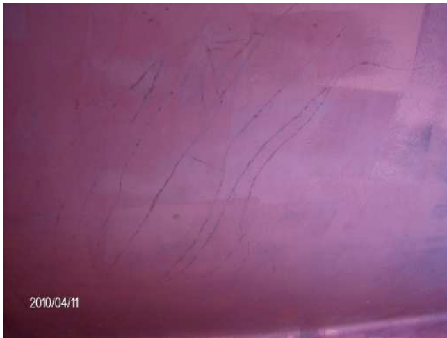
C1 gel coat crazing on the hull bottom. This area is approx. 12 square inches
