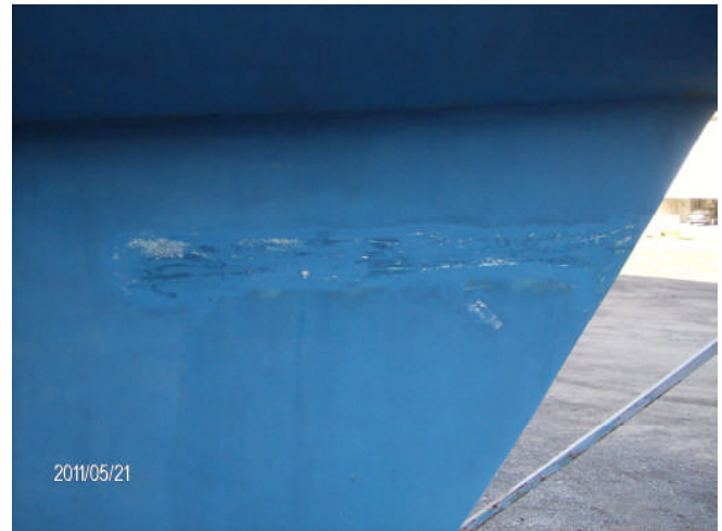
B1 signs of water leaking at the hull to keel joint
