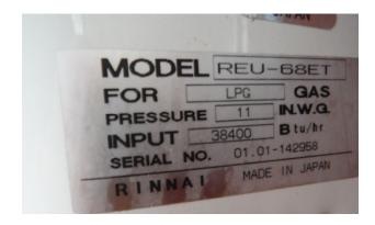
Just came across this propane water heater in a sloop. It's flueless, which means the CO produced does not vent outboard of the vessel. ABYC A26 states unattended appliances incorporate a room sealed combustion system. This heater does not.
